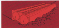
8. Reef concrete is placed to add strength and rigidity and the double-hulled tubes are side-launched for the 12-hour tow to the outfitting pier near Fort Myer.
