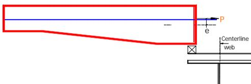
The longitudinal and transverse post-tensioning over the thickened negative moment areas of the slab also produces an eccentric pre-compression moment that increase the level of pre-compression at the top of slab, significantly increasing the effectiveness of the post-tensioning in controlling tensile stresses due to live load
